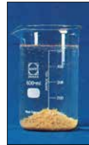
Clear water with flocculated matter
